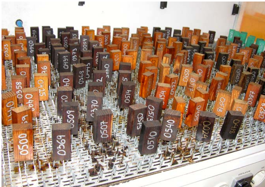
Figure 1. Drying of tar-coated test specimens in ventilation cabinet with UV-light.
