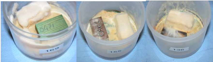
Figure 4. Treatments that seemed to cause strong inhibition of Gloeophyllum mycelium growth. Copper-naphthenate reference on the left, Kiln tar 4 in the middle and Retorte tar 4 on the right.
