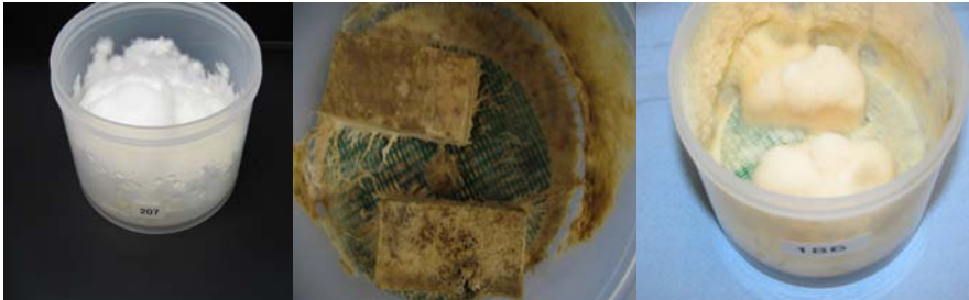
Figure 3. EN 113 vessels after test. Poria placenta on the left, Coniophora puteana in the middle and Gloeophyllum trabeum on the right.
