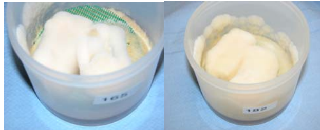
Figure 8. Further treatments that did not seem to cause any inhibition of Gloeophyllum mycelium growth. Retorte 4 coated roof shingle on the left and Servalac on the right.
