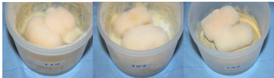
Figure 7. Treatments that did not seem to cause any inhibition of Gloeophyllum mycelium growth. Retorte tar 1 on the left, Retorte 2 in the middle and Retorte 3 on the right.
