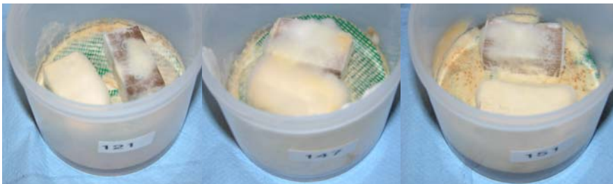
Figure 5. Treatments that seemed to cause slight inhibition of Gloeophyllum mycelium growth. Kiln tar 1 on the left, Kiln tar 2 in the middle and Kiln tar 3 on the right.
